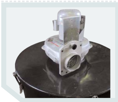
CLOSE-UP OF BLOWER WITH ADJUSTABLE DAMPER
